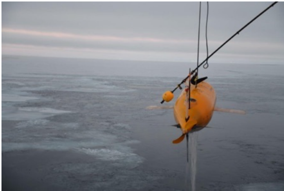
Figure 1. Autosub Long Rang under ice exploration.
