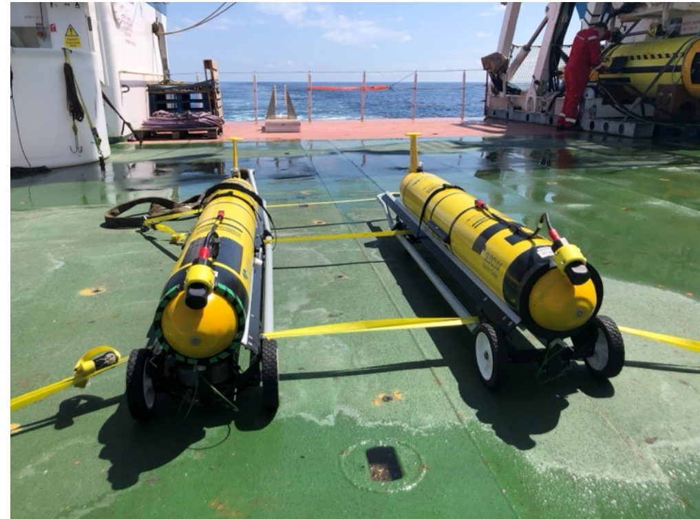
Figure 18. BSD Gliders 305 and 330 onboard RRS Discovery before open-water missions.
