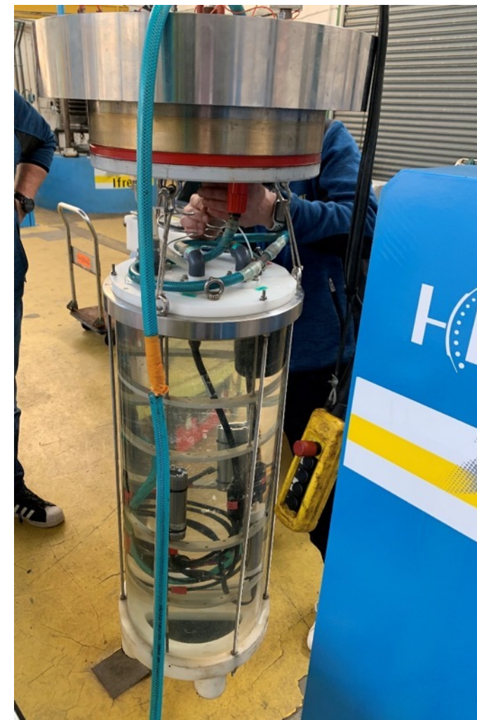
Sensor installation in the hyperbaric chamber
