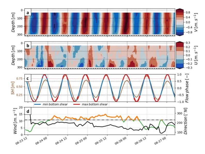
Fast tidally-driven flows  $\pm 1.2 \text{ m.s}^{-1}$  along strait primary flows  $\pm 0.3 \text{ m.s}^{-1}$  cross strait secondary circulation
