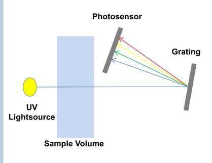
Wide spectrum UV light is emitted by a lamp and collineated to form a beam.
