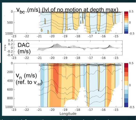
Depth Average Current (DAC) is estimated from the end-dive dead reckon position (from the flight model) and the end-dive GPS positioning.
