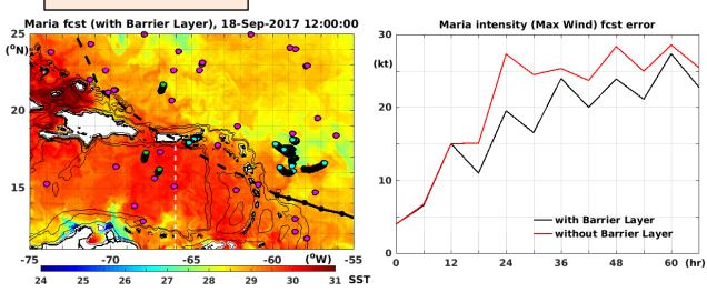
In <u>black</u>. intensity when the ocean model assimilates all observations. In <u>red</u>, when the ocean model misses the barrier layer. rms intensity error for Hurricane Maria (2017) is reduced with the assimilation of the barrier layer.
