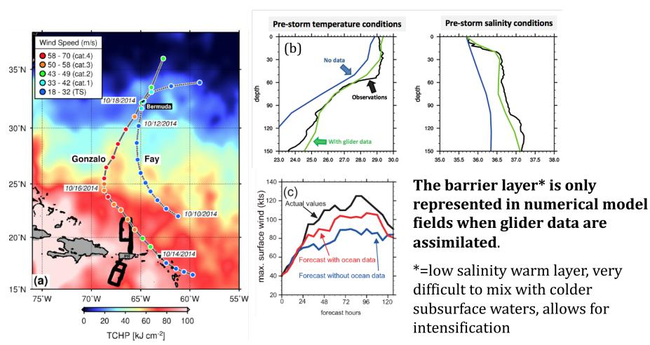
Assimilation of underwater glider data along with other ocean observations reduced the error on Hurricane Gonzalo intensity forecast by approximately 50% using the next generation ocean-atmosphere coupled HYCOM – HWRF model.
