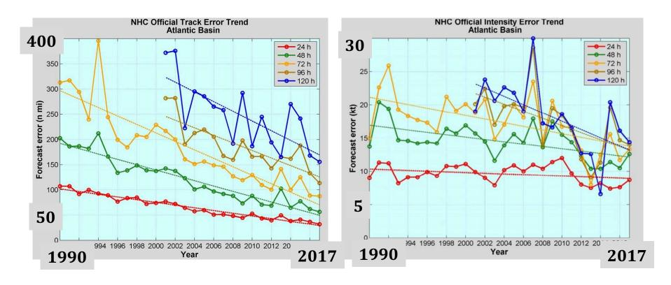
In average, error in intensity forecast has remained almost unchanged (for 48hs or less forecasts) and larger than 15 knots (for 72hs or more forecasts) during last 25 years.
