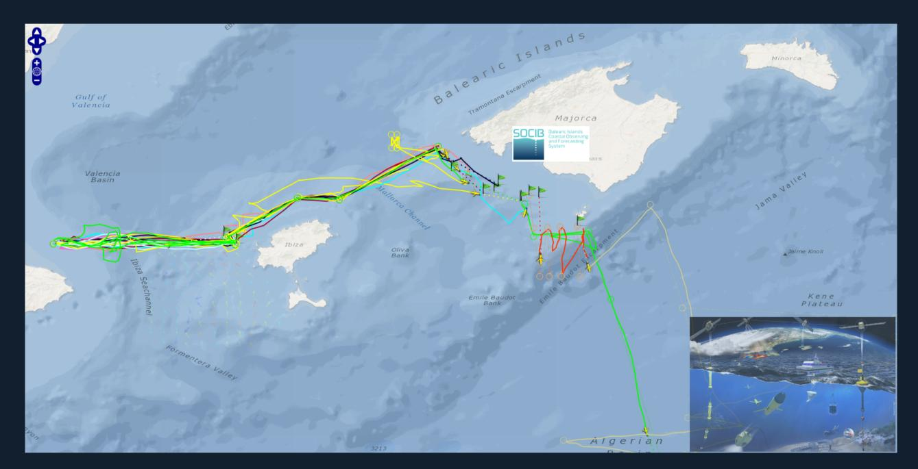
Quasi-continuous glider missions have been carried out in the Ibiza Channel since 2011 to better understand the mesoscale variability in the Balearic Channels (Heslop et al., 2012). Since then:
