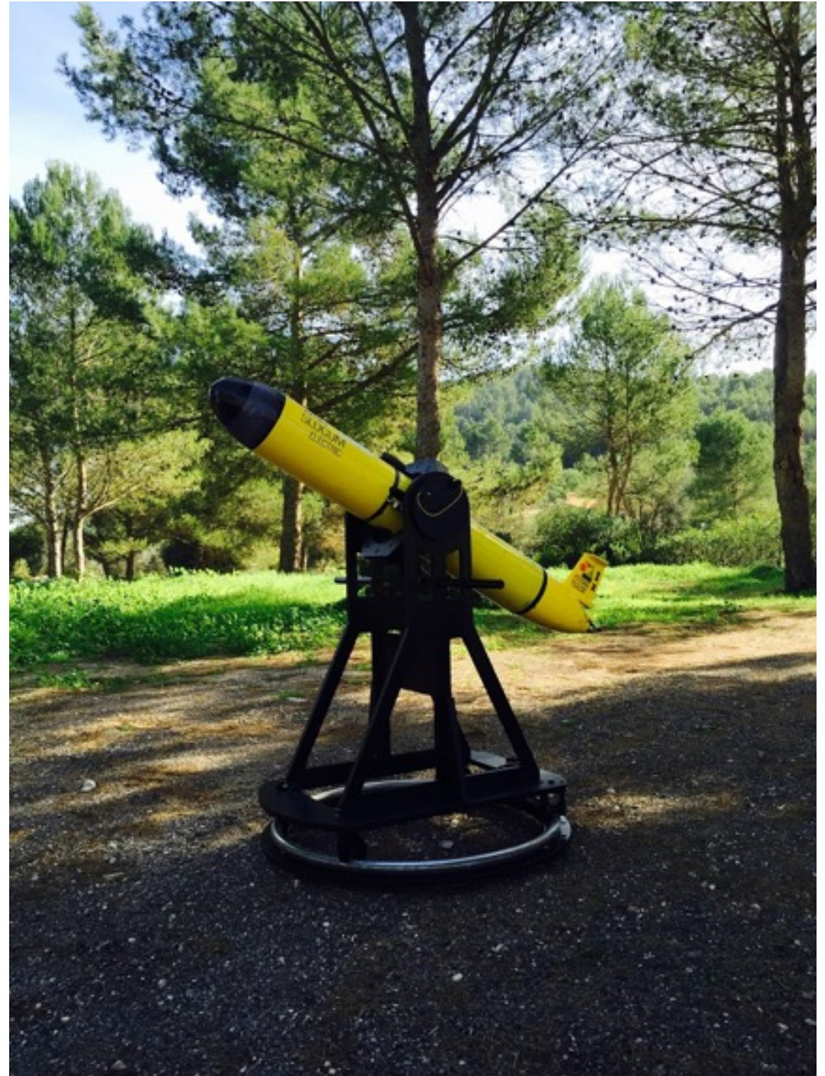
Cradle for compass correction procedure (SOCIB)
