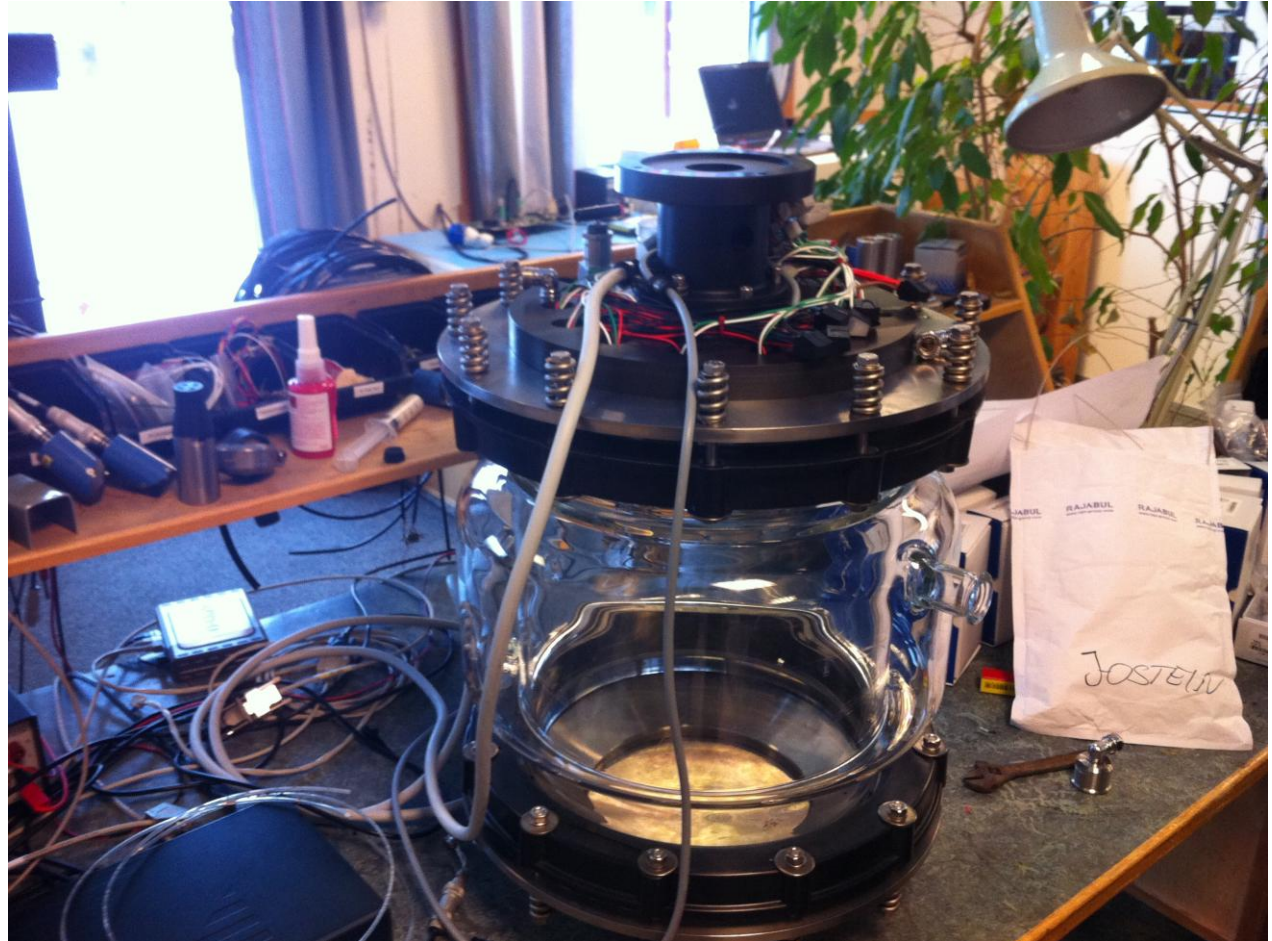
Elaborate calibration facility for O_2 and pCO_2 under construction
