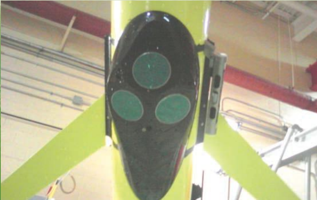
A 400 kHz Nortek Aquadopp Profiler mounted on the underside of a Webb Research Slocum glider operated by researchers at Memorial University
