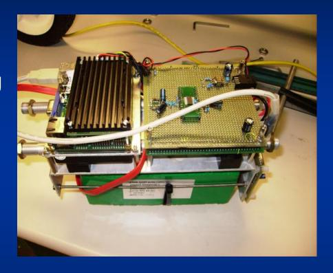
Intel® Atom™ Z530 @ 1.6 GHz, 512MB DDR2 533 MHz, Gb Ethernet, 1 TB SATA SSD
